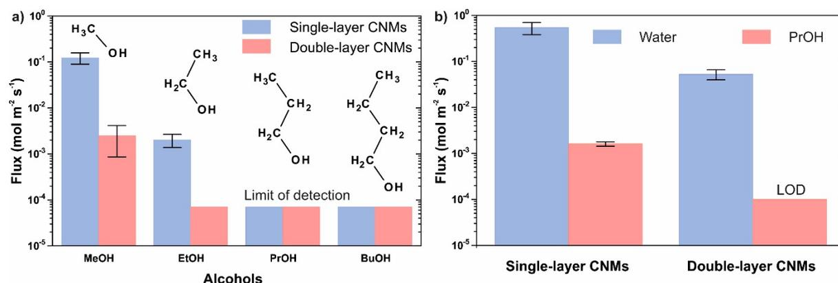
Figure 2. a) Transmembrane flux of pure alcohols in single- and double layer CNMs under saturation vapor pressure [3]. b) Transmembrane flux of D<sub>2</sub>O and C<sub>3</sub>H<sub>7</sub>OH in single- and double layer CNMs upon exposure to the azeotropic mixture [3].
