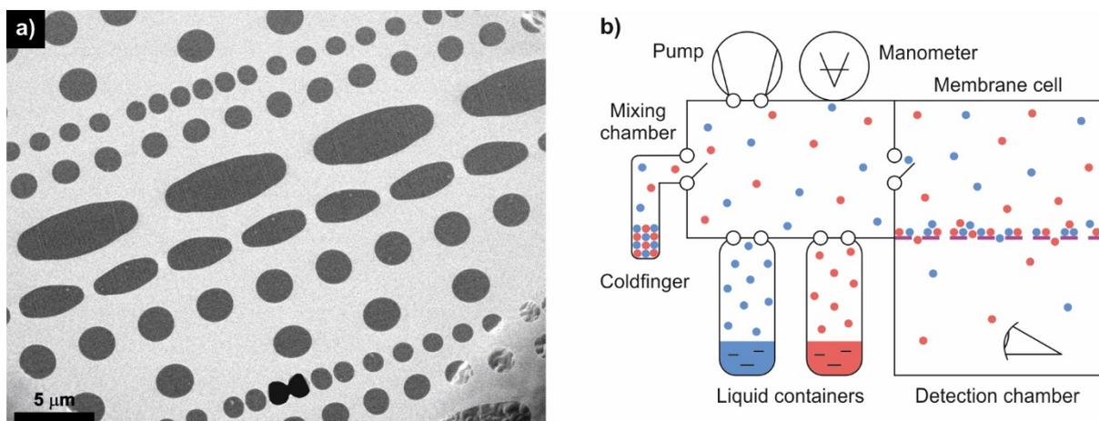
Figure 1. a) Helium ion micrograph of a large area TPC CNM suspended over a TEM grid [1]. b) Schematic of the ACP measurements with vaporous mixtures [2].
