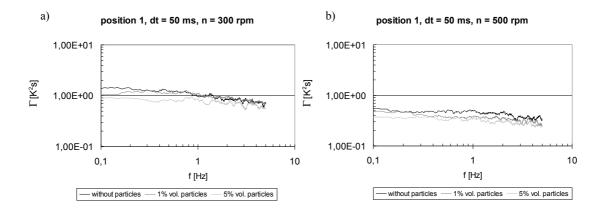
Figure 3: Temperature spectra for flow with and without particles. a) n=300 rpm, b) n=500 rpm
