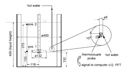
Figure 1: Experimental set-up
