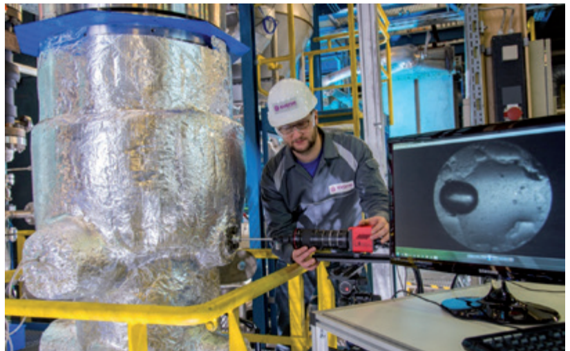
Fig. 108: Testing a laser endoscope used for determining bubble size
