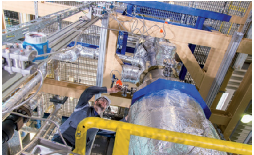
Fig. 107: Pressurised bubble column reactor at a technical centre operated by Evonik Industries AG
