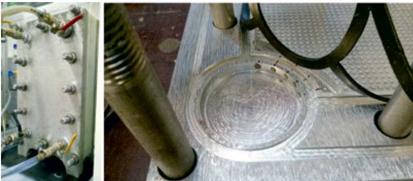
Abb. 95: Left: Demonstrator in operation; Right: Base plate showing the gasket and the studded surface that supports the film
